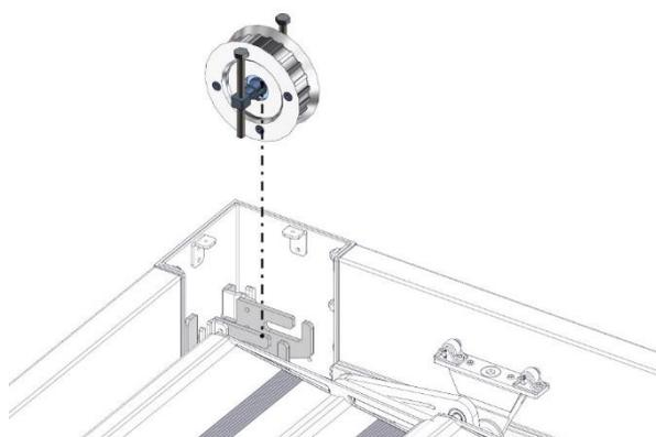
3. Turn and place the stretching bolts. The stretching bolts must be placed in the related housing.
