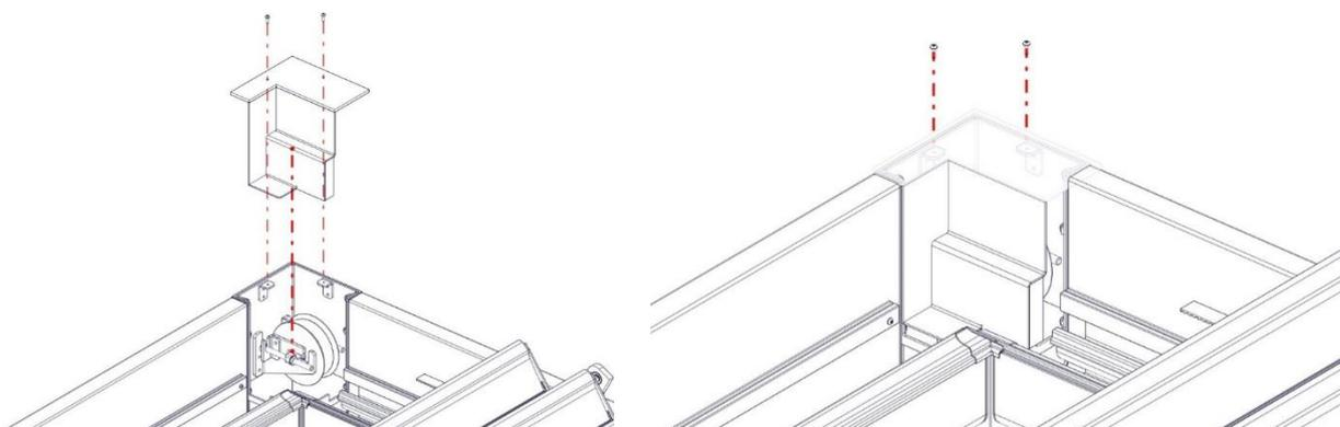
**3. Place the tubular Motor covering profile; This profile should be on the rear and fixed with M2,9x13mm screws. If there is perimeter lighting, the lighting control box should be placed on the profile as you see at below. The cables should go from the corner to the box.**
