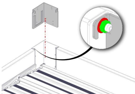
2. Place the front gear into the 'front mechanism house'.
