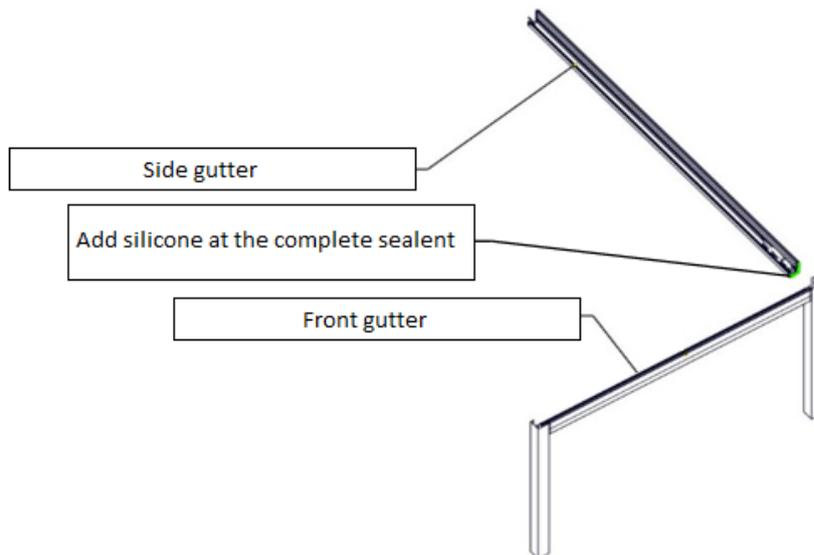
4. Fix the lateral side integrated gutter to the rear integrated gutter with M10 Sealed Nuts.
