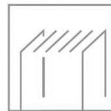
7. Install the front cover profile. Now mount the corners. Seal the opening seams with silicon sealant.
