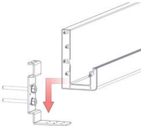
4. Fasten the wall mounting bracket cover on top and tighten it with M8x25mm bolts.
