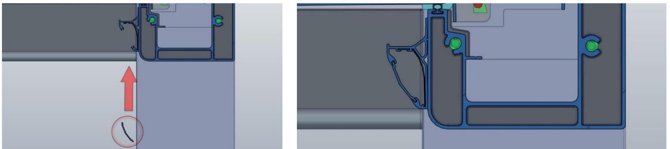
**3.** Place the corner plastic between the perimeter lighting profile in the corners.
