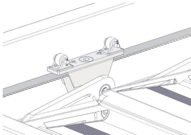
**3. Rail belt stretching; This bolt ensures the tension on the belt is adjustable**
