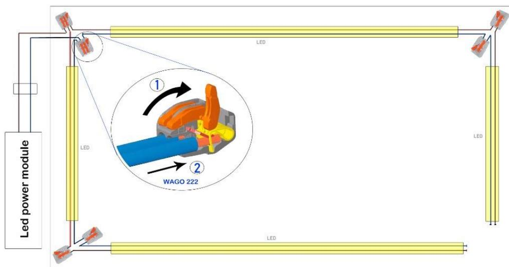
**⚠** Tip: The wires to the LED lighting are soldered and therefore more fragile on the solder point, do not pull or bend intensively at the installation.
