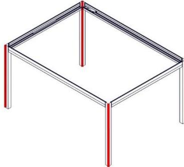
Check the lateral gutters level
