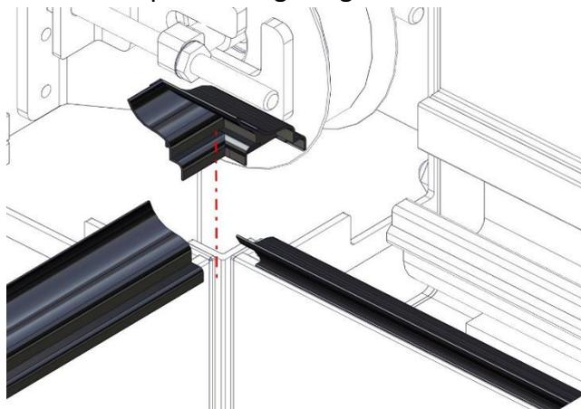
**2. The corner cap should be on the frontside. Fix it to the housing with the M2,9x13mm rounded head screws.**
