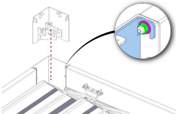
7. The bracket's housing will fit exactly on the pins. After that place the washer and fasten the nuts.
