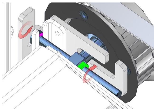
**4. Make sure there is the same stretch level of the belt on both sides. It should be just so tight that it just doesn't sag. Do not tighten.**
