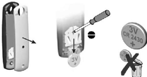
Using a small screwdriver loosen the screws on the reverse side of the remote control and remove the back cover. Replace the battery with one 2430 Lithium 3V Battery.
