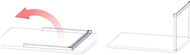
3. Connect the integrated gutter and lateral integrated gutter in a position as shown at below figure.
