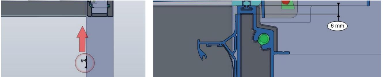
**2.** Place the perimeter lighting profile cap to the housing on the perimeter lighting profile.
