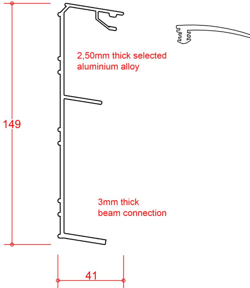
Aluminium wall profile cover cap for seamless wall connection
