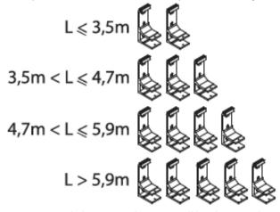
It is recommended to mount the outer wall brackets at a distance of 20 to 45 cm from the ends of the awning, and place the remaining brackets at equal intervals.
