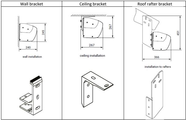
Note: After installation the casette has a slight inclination from the vertical.
