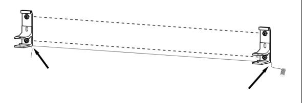
10) Slide the awning (cassette) on wall brackets so that the construction is maximally pressed to the back (Note – before placing the awning verify the alignment of brackets – wall surface should be of the same thickness at installation spots).
