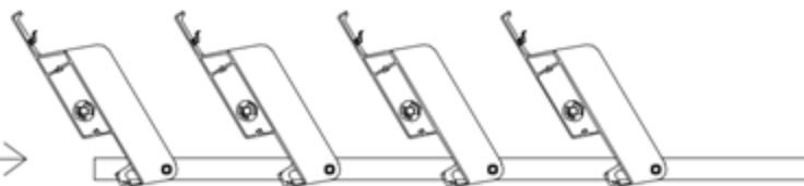
Fig. 2. Standard blade opening direction setting on Pergola SB350
